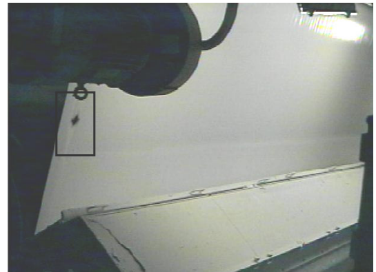
Figure 2.2. 1 st Coater DS (Showing Defect)
