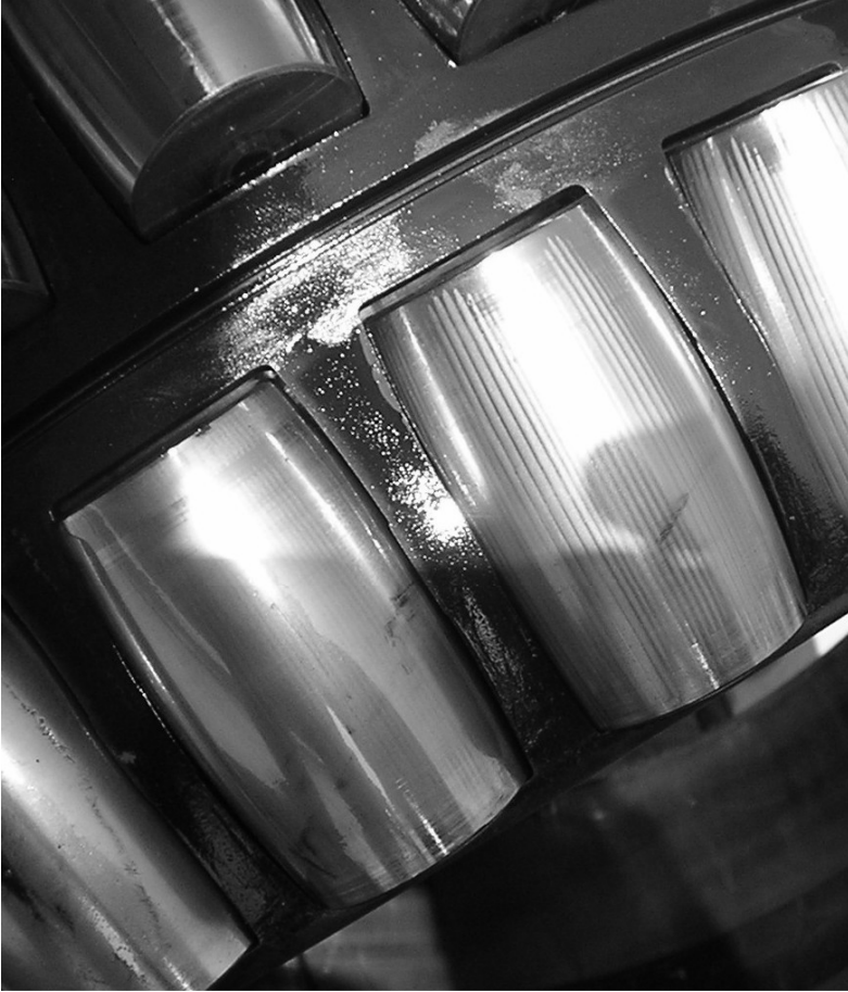
Photo showing the 'Washboard' effect on the Rollers (not all rollers).
